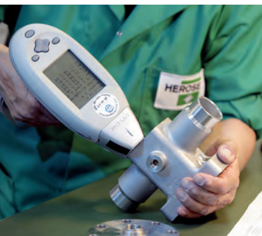
Material analysis and identification during the incoming goods check
